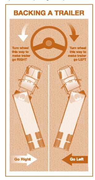
Figure 6.5 Backing a Trailer
