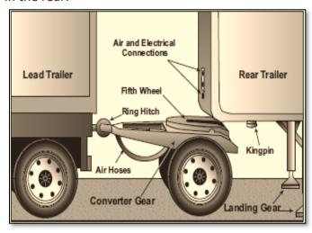
Figure 7.1 Converter gear on a dolly
