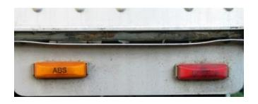
Step Two: Check that all external lights and reflective equipment are clean and functional.
