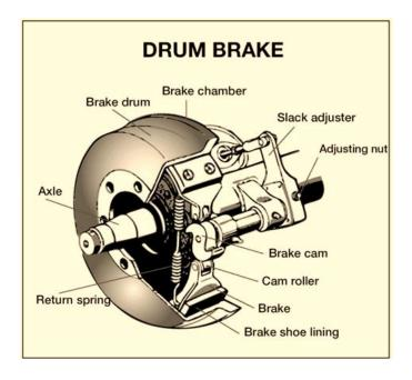
Figure 5.2 Drum Brake
