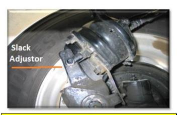
Special Note: The following are two (2) types of slack adjusters found in most air brake systems:
