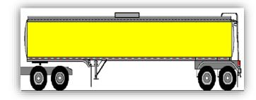
Be extremely cautious (slow and careful) in driving smooth bore tanks, especially when starting and stopping.
