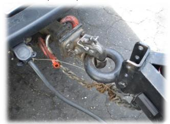
**Tongue or Draw-bar:** Trailer component attaching the truck to the trailer.
