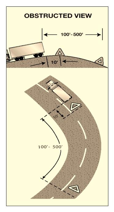
Figure 2.10 Obstructed View Triangle placement
