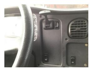
**Trailer Brake Handle in Freightliner Tractor**
