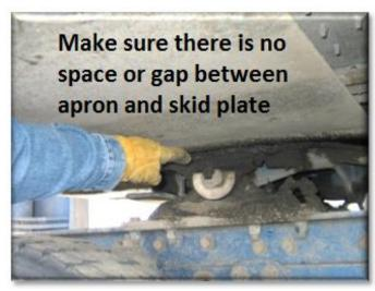
☐ Make sure there is no space between the apron on the trailer and the fifth wheel skid plate. If there is space, something is wrong (kingpin may be on top of the closed fifth wheel jaws, and trailer would come loose easily).
