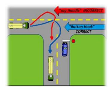
Figure 2.13 Correct Execution of Right Turn
