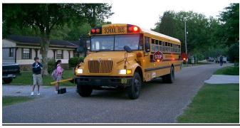
These lights warn applicants that the bus is stopping to load or unload students. 7" diameter lights are located in upper corners on front and back of bus. Inside lights are amber. Outside lights are red.
