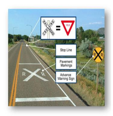
**Figure 10.6 Pavement Markings**
