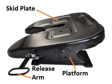
Release Arm (Fifth Wheel) releases fifth wheel locking jaws so that the trailer can be uncoupled. The release arm must be in the <u>engaged</u> position with locking jaws completely closed around the kingpin when pulling a trailer. This will prevent loss of the trailer during travel.
