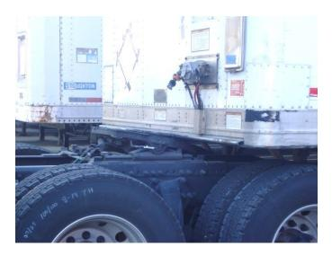
☐ Check that the kingpin and fifth wheel are aligned.
