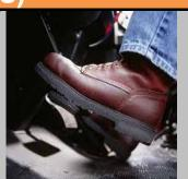
If equipped with a hydraulic brake reserve (backup) system, with the key off, depress the brake pedal and listen for the sound of the reserve system electric motor.
