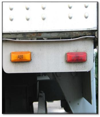
Figure 6.7 - ABS Malfunction warning Light.
