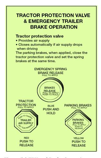
Figure 5.3 TPV and Brake Operation
