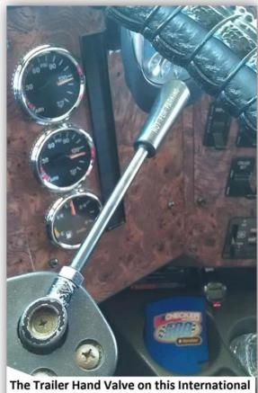
The Trailer Hand Valve on this International tractor is located on the steering column. Figure 6.5.A
