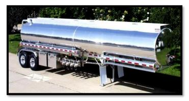
Fuel Trailer with bulkheads can carry different grades of fuel
