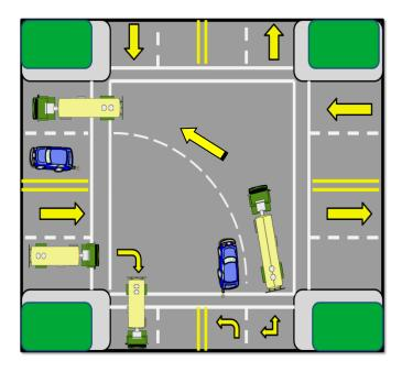
Figure 2.14 Correct Execution of Left Turn
