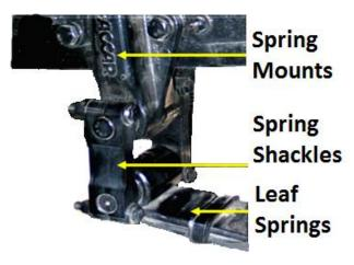
Damaged or missing leaf spring parts may lead to a loss of control or a rollover if the vehicle falls on the frame or on a tire. Shifted springs may strike a tire, causing a blowout or interference with steering.
